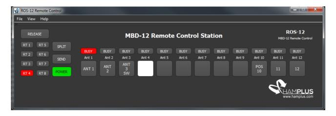
On the picture above, the ROS-12 UI shows that the MBD-12 is commuted at Antenna 4, Antenna 1 is currently busy (cannot commute to busy positions) and also shows that Rotor 4 is ON.
