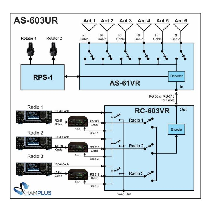
Diagram of blocks and connections of the antenna switch **AS-603UR** <u>without</u> the rotator power supply module, mounted in two cabinets
