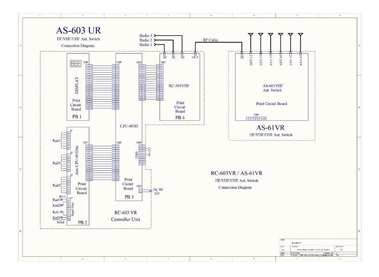
Diagram of the blocks and connections of the antenna switch **AS-603UR** <u>with</u> the rotator power supply module, mounted in three cabinets
