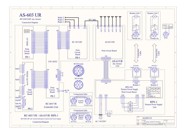
Diagram of blocks and connections of the antenna switch  $AS-603UR \underline{with}$  the rotator power supply module, mounted in two cabinets
